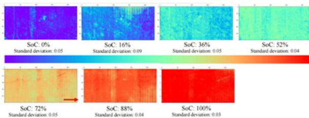
**Figure 5:** SOC uniformity change of fresh battery during charging.
