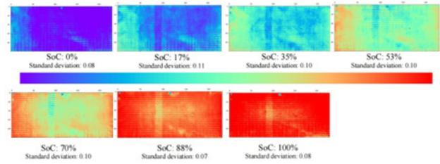
**Figure 6:** SOC uniformity change of cycled battery during charging.
