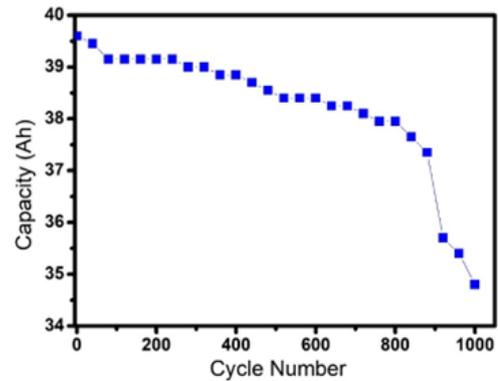
Figure 2: Cycle performance of the battery sample.
