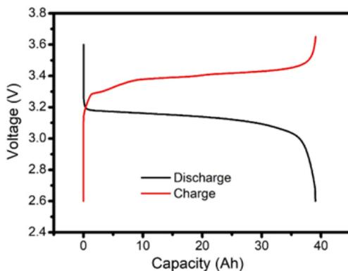
Figure 1: Charge-discharge characteristic curve of the traction battery sample.
