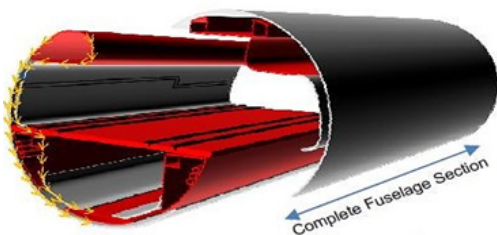
Figure 8: Thermoplastic composite fuselage section [18].
