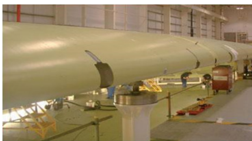
Figure 14: A380 Welded fixed wing leading edge from PPS [27].
