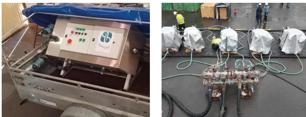
Figure 5: A trailer-mounted Vulcan-500 NB generator on the left, alongside a quintet of such weather-shielded (IP-68) and skid-mounted generators connected to a flow manifold for mass oxygenation and carbonation of crop-spray and irrigation water for, inter alia, soil-regeneration trials, also using parallel administration of NB-cultivated microalgae.
