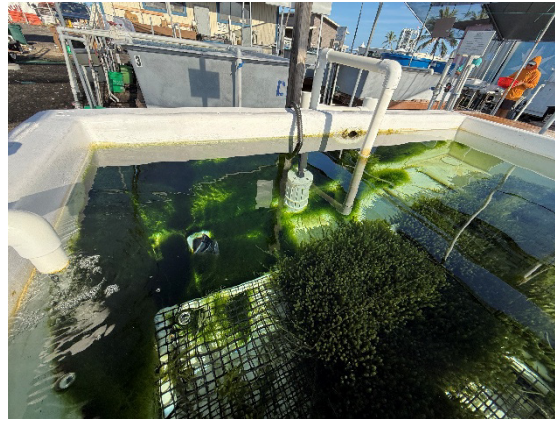
Figure 6: Enhanced growth of Ulva species of macro-algae by air nanobubbles around the submersible NB generator – see the green film.
