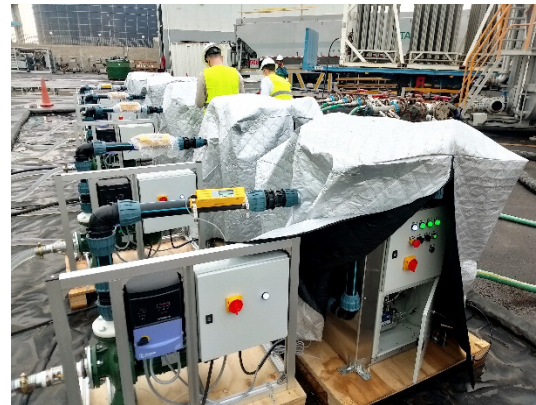
Figure 1: Side-views of one/multiple 1,000-l.p.m. water-flow model of “Vulcan-500” nanobubble generators, with inlet- and outlet-manifold piping and pump arrangements. Mass-flow controllers are installed for controlling of gas flow, with variable-speed drives on the water/aqueous pumps for liquid-flow control, and settings for ratio control of liquid to gas (and subsequent nanobubble formation).
